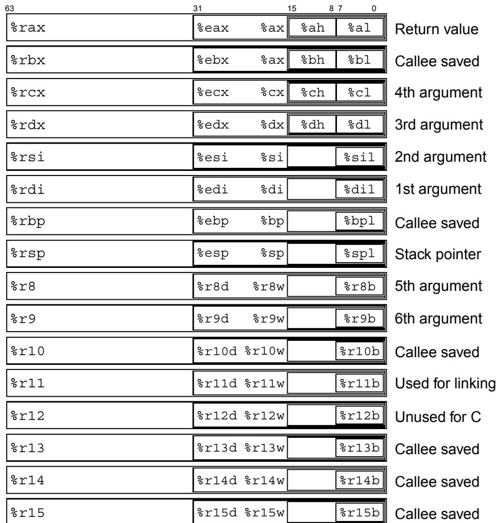
Figure 2: **Integer registers.** The existing eight registers are extended to 64-bit versions, and eight new registers are added. Each register can be accessed as either 8 bits (byte), 16 bits (word), 32 bits (double word), or 64 bits (quad word).
