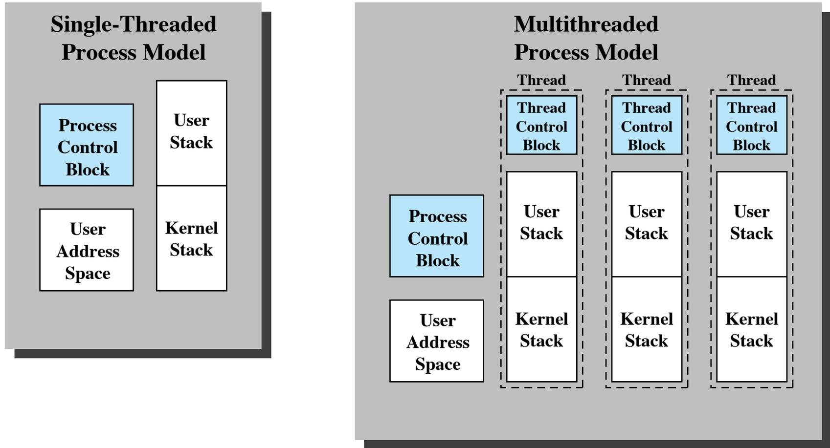
**Figure 4.2 Single Threaded and Multithreaded Process Models**
