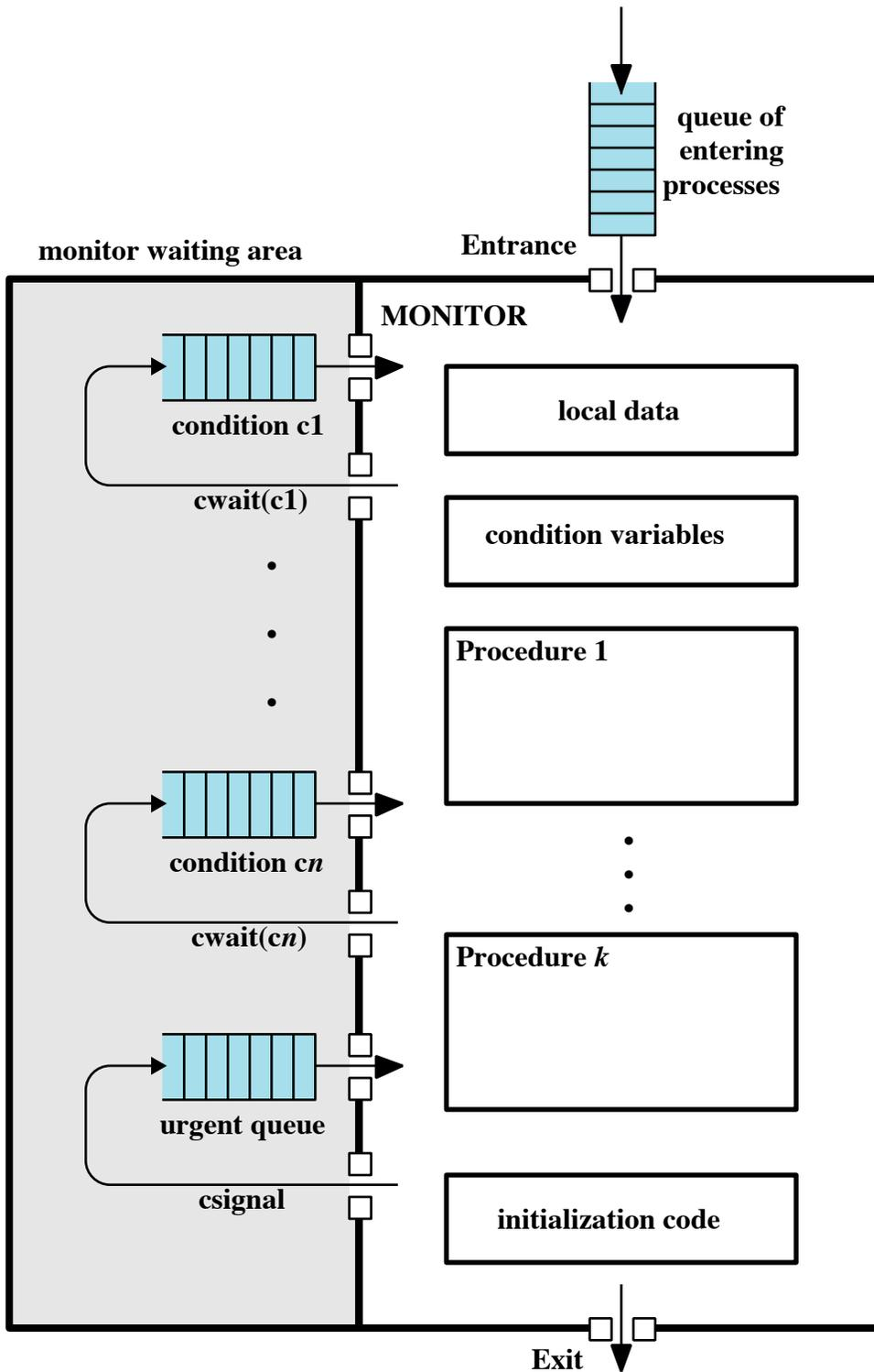
**Figure 5.15 Structure of a Monitor**
