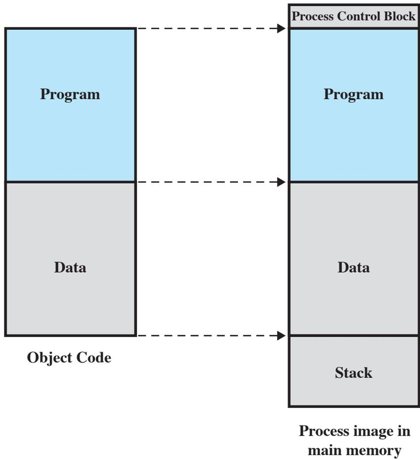
**Figure 7.13 The Loading Function**
