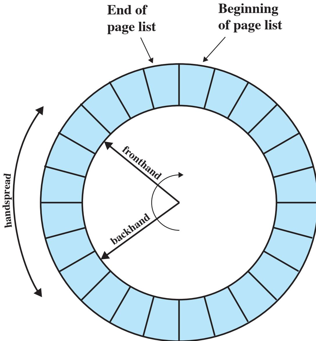
**Figure 8.23 Two-Handed Clock Page-Replacement Algorithm**
