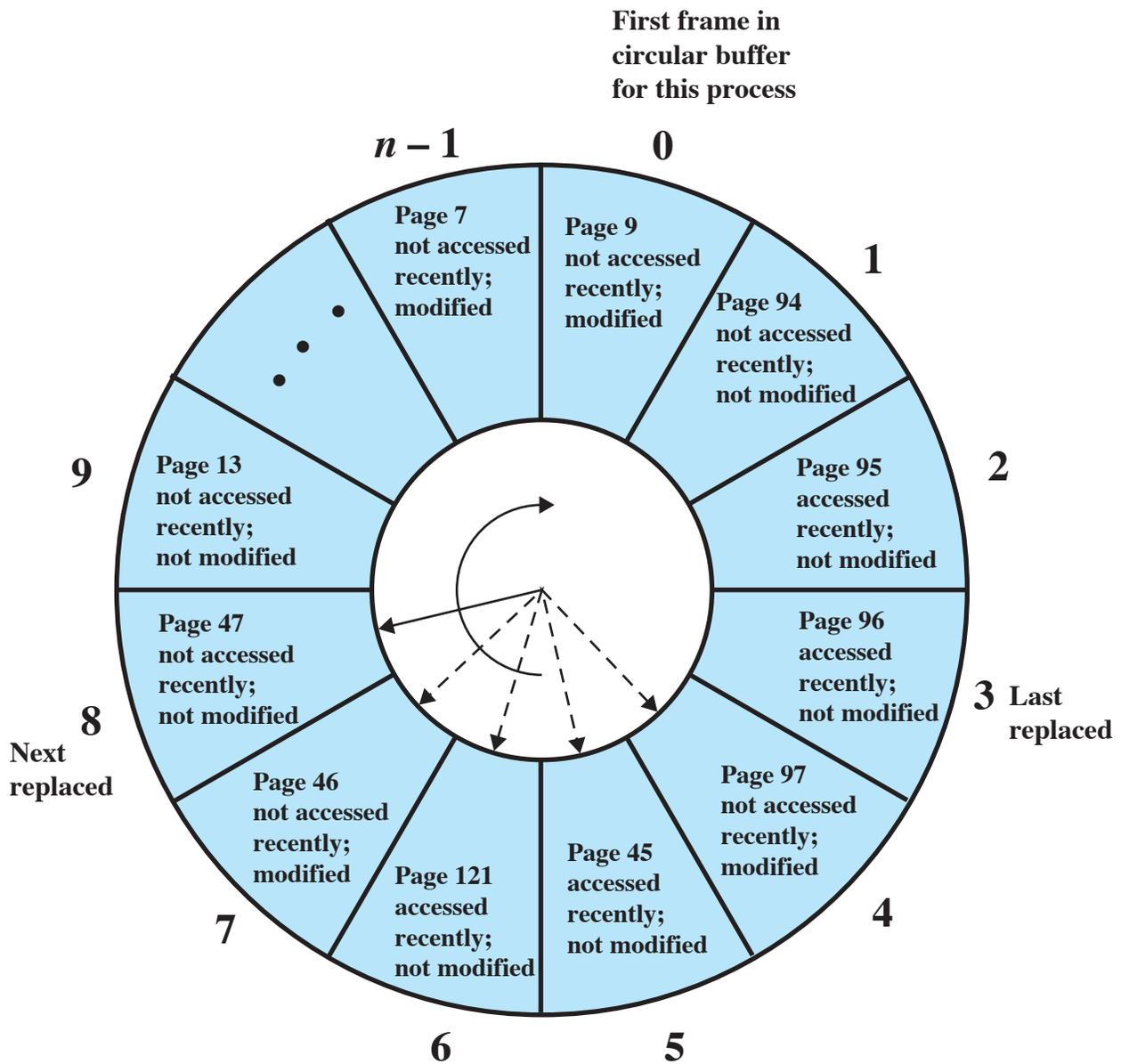
**Figure 8.18 The Clock Page-Replacement Algorithm [GOLD89]**
