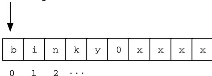
The memory drawing shows the local variable `localString` with the string "binky" copied into it. The letters take up the first 5 characters and the `\0` char marks the end of the string after the 'y'. The x's represent characters which have not been set to any particular value.
