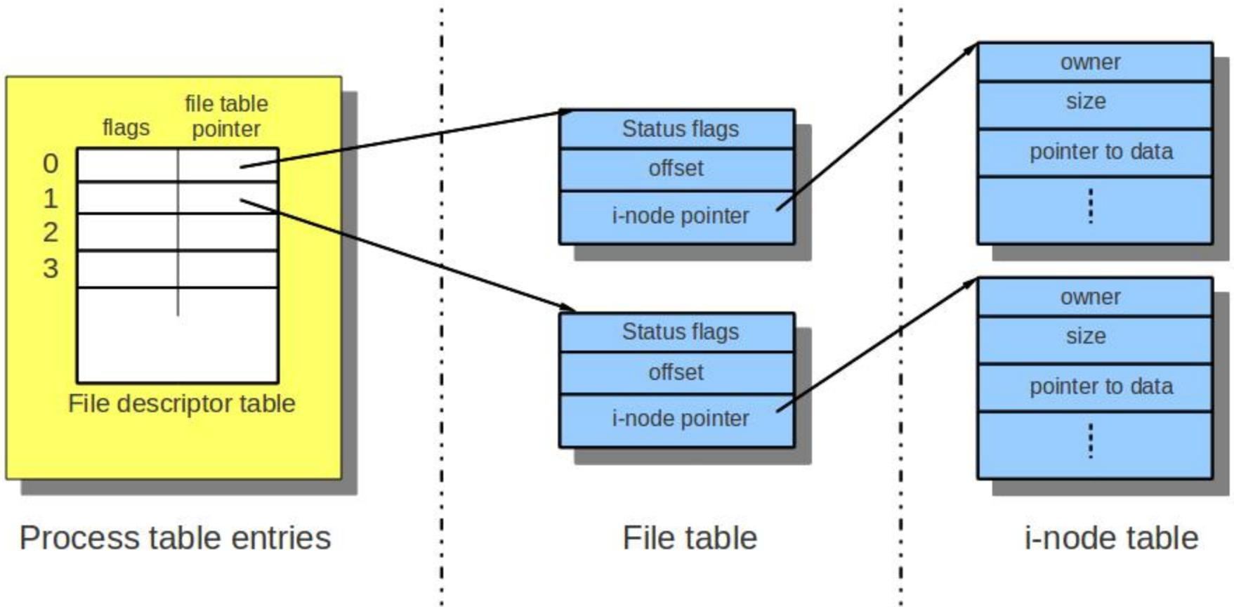
**Fig. 1. Kernel data structures for open files**
